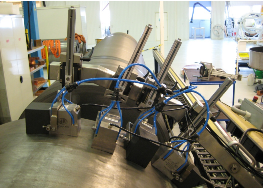
Figure 6-19. Fixture with four 32-element linear arrays (1.7 MHz) for ultrasonic testing of the outer five centimetres with shear waves and approximately 70° incident angle.
