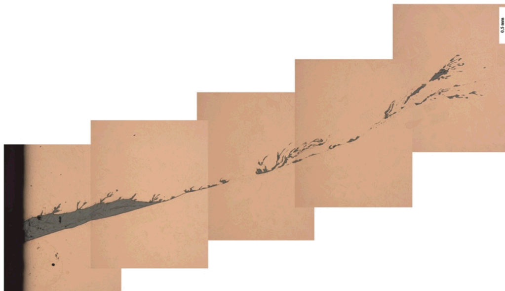
Figure 7-34. Metallographic cross-section of a forging lap extending from the bottom surface (left). The depth was measured to about 8 mm.
