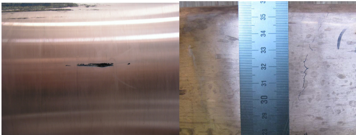
Figure 7-27. Manufacturing defects in copper tubes. The left image shows an axial scratch (T46) in an extruded tube and the right image shows a crack-like defect in a pierce-and-draw tube (T83).
