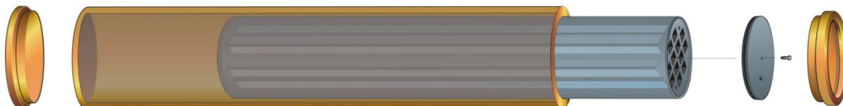
Figure 3-1. SKB reference canister with an outer corrosion barrier made of copper and an insert made of nodular cast iron.
