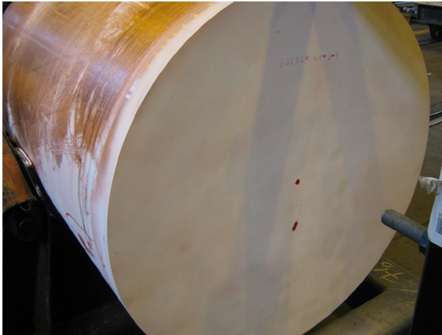
Figure 6-35. Dye penetrant inspection results on the end surface of a machined copper tube ingot. In the centre, two penetrant indications are visible.
