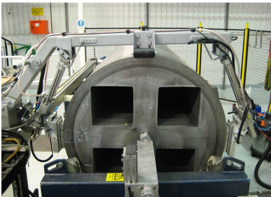
Figure 6-23. Ultrasonic testing of the volume between the channel tubes in a PWR insert using the Posiva probe fixture.
