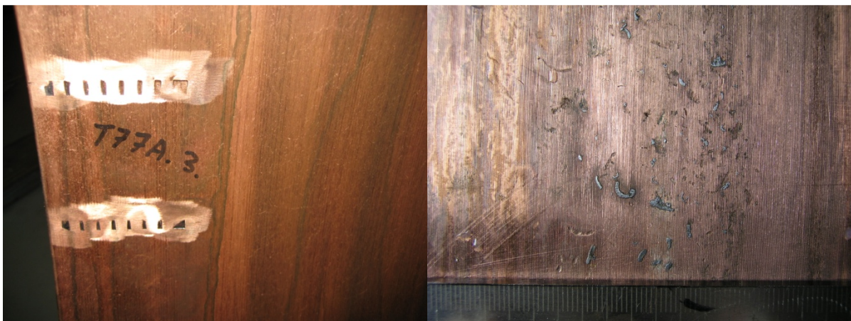
Figure 7-26. Handling defects manifested as indentations on the inside of tube T77 (left) and foreign material on the outside of tube T43.
