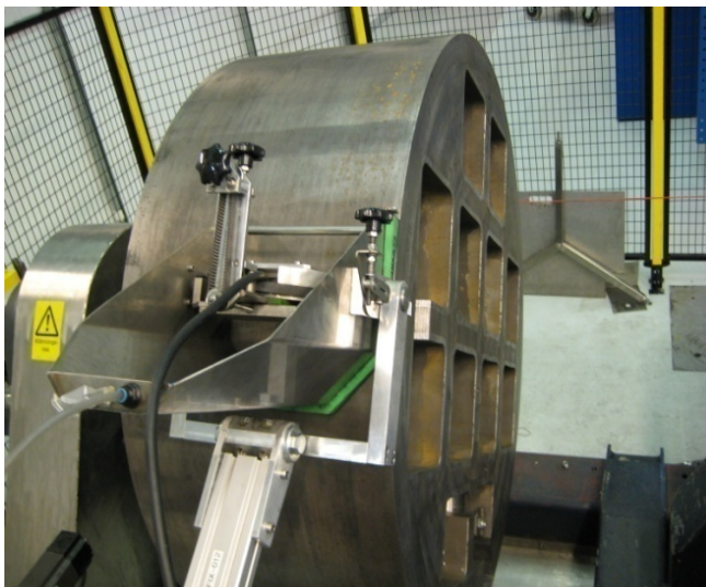
Figure 6-8. Linear array for local immersion inspection of the cast iron insert.
