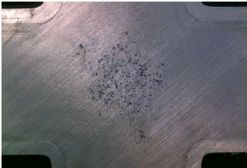
Figure 7-6. Photograph of the shrinkage pores indicated in Figure 7-5 between the fuel channels in a PWR insert.
