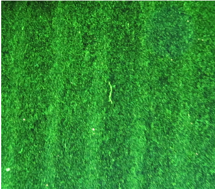
Figure 7-16. MT-1, a 3-mm linear indication obtained by magnetic particle inspection. The indication detected on the envelope surface of the insert is oriented in the circumferential direction. The five broader, weaker, non-relevant indications along the entire figure in the same vertical direction of the figure are caused by magnetic leakage fields related to the surface finish left by the turning operation.
