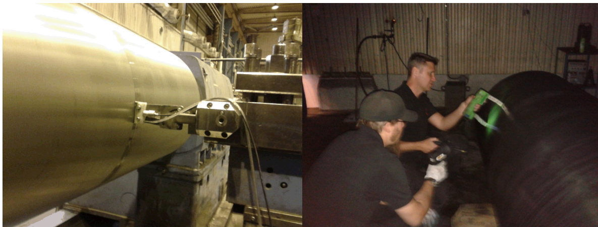
Figure 6-7. Ultrasonic and magnetic particle inspections of the inserts are performed by the supplier. The ultrasonic inspection (left) is automated using a turning machine as the manipulator; the cutting tool has been replaced with an ultrasonic probe that is fed with water as a couplant. The fluorescent magnetic particle inspection (right) is performed by magnetising each square decimetre of the insert in two orthogonal directions under UV lighting.
