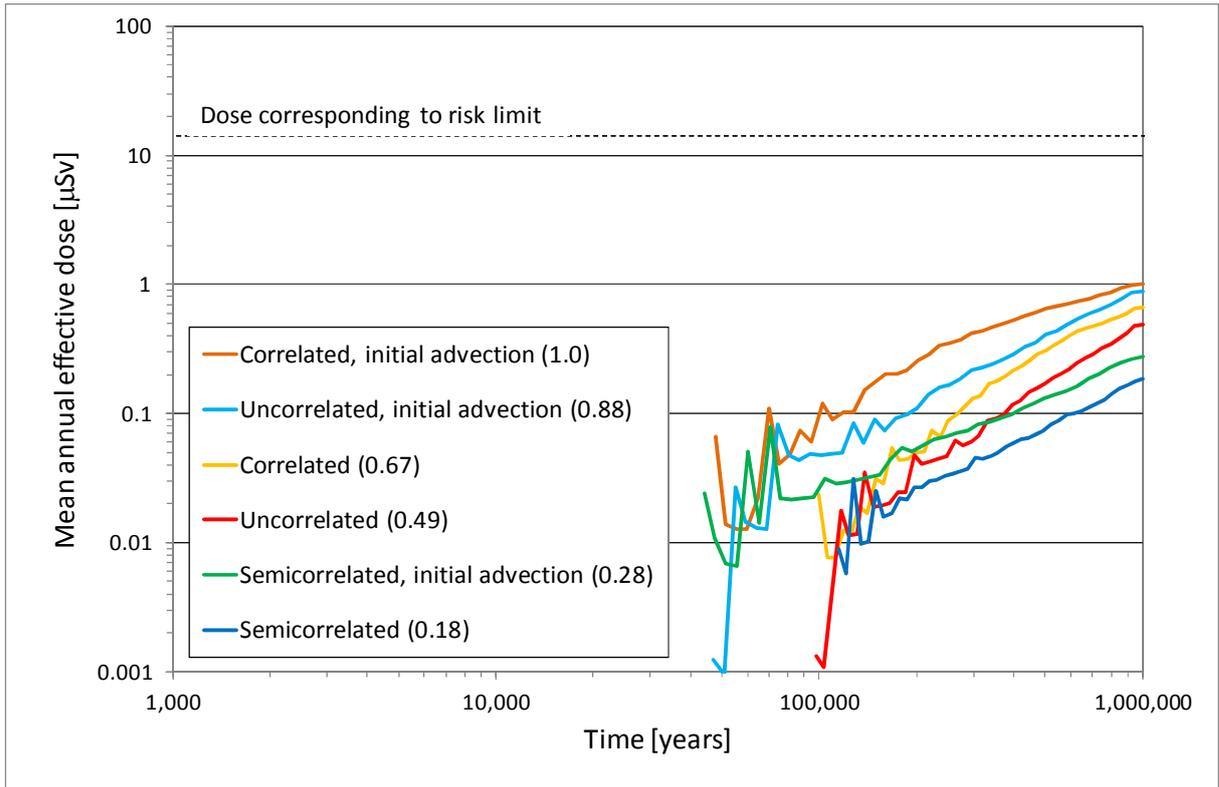
**Figure 1.** Far-field mean annual doses for analytical, probabilistic calculations of the six corrosion variants of the corrosion scenario, i.e. the six cases in Table 1 when using Equation (9a). The peak doses are given in parentheses in  $\mu\text{Sv}$ . (Figure 13-42, p. 689 in TR-11-01.)
