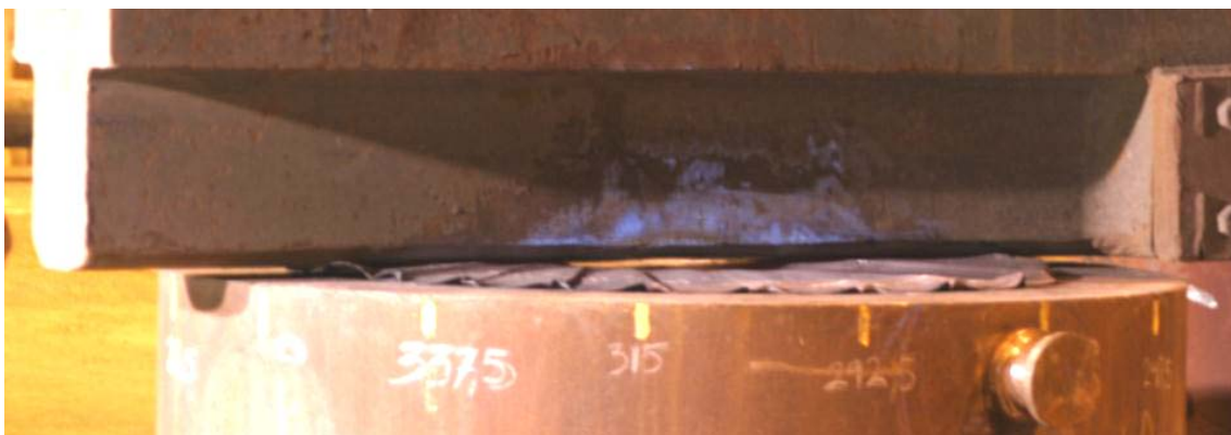
Figure 1-4. Cogging with tools and workpiece shown.
