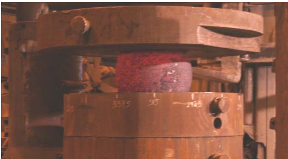
Figure 1-1. Upsetting of the workpiece in the reference process.
