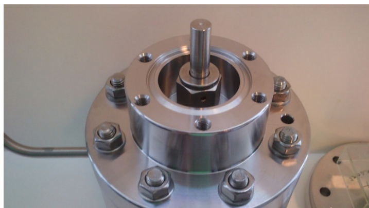
Fig.2-3. The new lid, here with blind VCR 1/4” connection together with the outer CF-38 seal.
