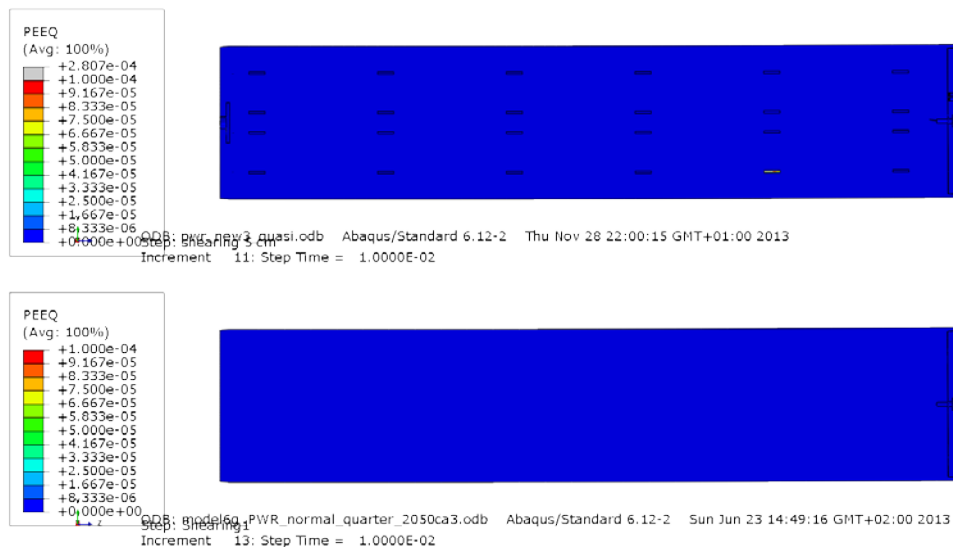
Figure A8-9 Plot showing plastic equivalent strain (PEEQ) for the insert after 5 cm shearing for detailed PWR model (top) and the reference PWR model (bottom).
