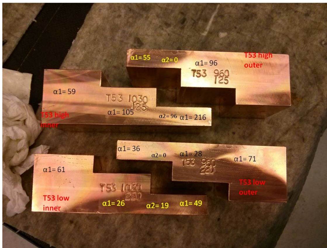
Figure 6-12. Step wedge test specimen from low and high attenuation regions in T53.
