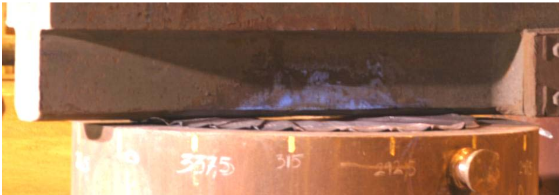
Figure 1-4. Cogging with tools and workpiece shown.
