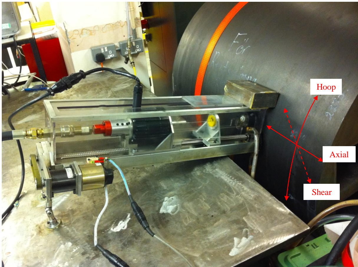
Figure 6: An image of the DHD machine during the gundrilling of measurement 1 with axes orientation illustrated.
