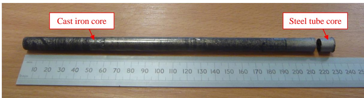
Figure 7: A photograph of the 3 mm cores removed from the location 2 measurement.
