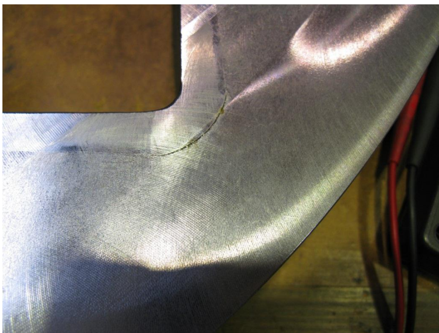
Figure A2:6 The PWR sample. The corner of space, molten material has loosened from the tube. Similar release was found close to space 3
