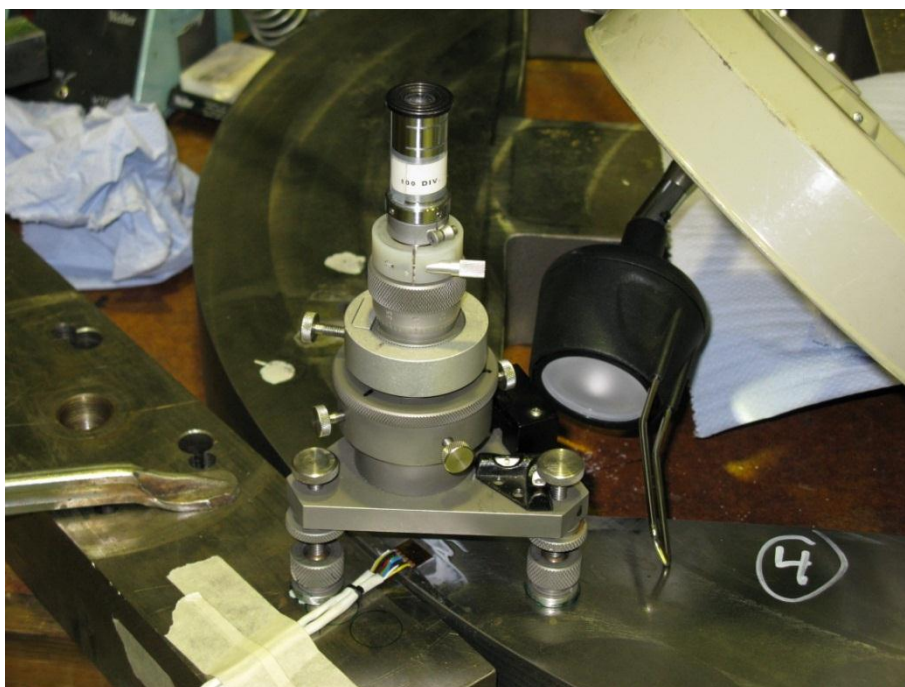
Figure A2:8 The hole drilling rig cemented to the PWR sample at space 4. As the hole should be drilled close to the outer edge of the sample the third foot of the rig had to be placed on a metal block lying close to the sample. As the block must be immovable, it was clamped to the work bench.
