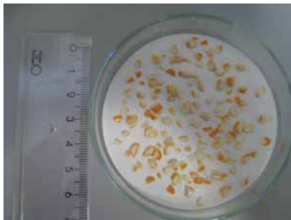
Figure 4-3. Orange surface 2 to 4 mm ThO 2 particles after crushing and flushing with isopropanol and ethanol.
