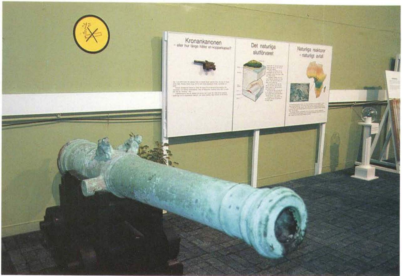
Figure 9-3. This is the natural analogue corner of the exhibition. The Kronan canon, salvaged after 300 years in the Baltic Sea, provides an interesting example of copper corrosion. The wall screens feature the Cigar Lake uranium deposit in Canada and the Oklo “reactors” in Africa. (Photo by Bengt O. Nordin.)
