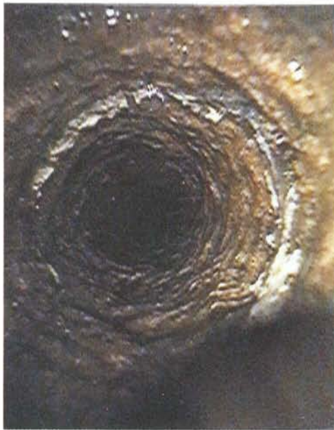
Figure 16-4. Hardcopies from videoimagescope survey in boreholes, showing: a) grouting materials in a fracture at 7.2 m depth in a borehole, b) point leakage of water (channelling) from a fracture into a borehole, at 15.2 m depth.
