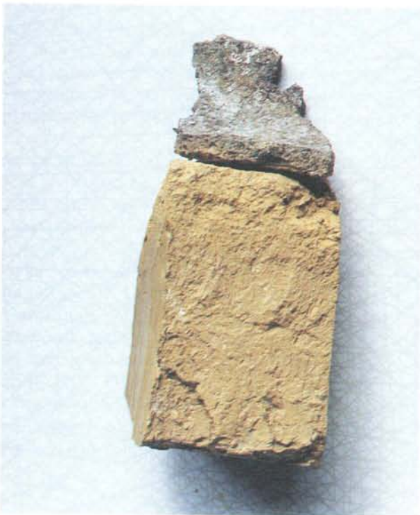
Figure 15-3. Part of clay closest to the heater from the 4 year test. The darker color of the clay in contact with the heater indicates the transformation into claystone. The thickness of this layer is 1 cm.
