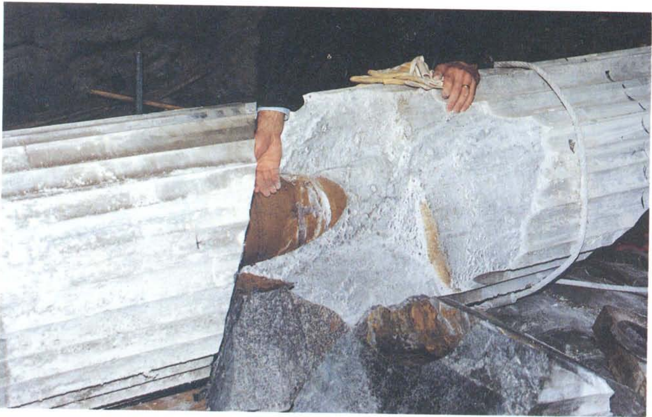
Figure 15-2. Heater and surrounding Fo-Ca clay after central part of the heater has been sampled. In order to extract the clay body the overcoring technique was used. The pipes of the slot holes, made in the rock, make the recovered piece look like a Greek or Roman temple column.
