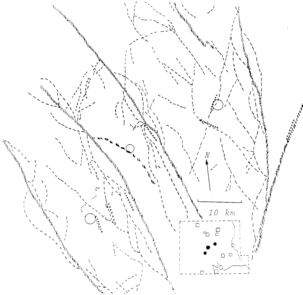
Figure 12b. The lineaments given by Henkel (1988) for the area of the three events of figure 12a. The dotted lines mark the lineaments having positions and strikes that fit the fault plane solutions.
