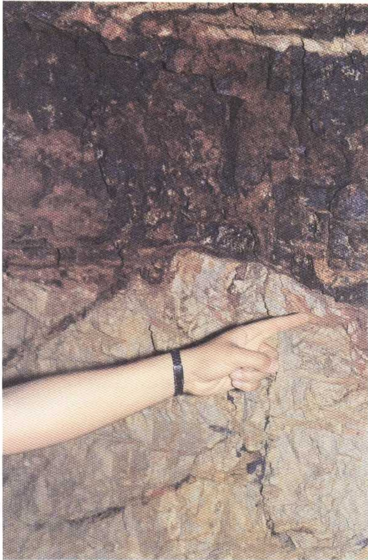
Plate 3. Magnetite dyke in the DNPM adit. The magnetite emplacement caused little contact effects on the host rock. Oxidation free zones can be found (lower right) due to the low permeability of the clays which constitute the groundmass of the host rock.
