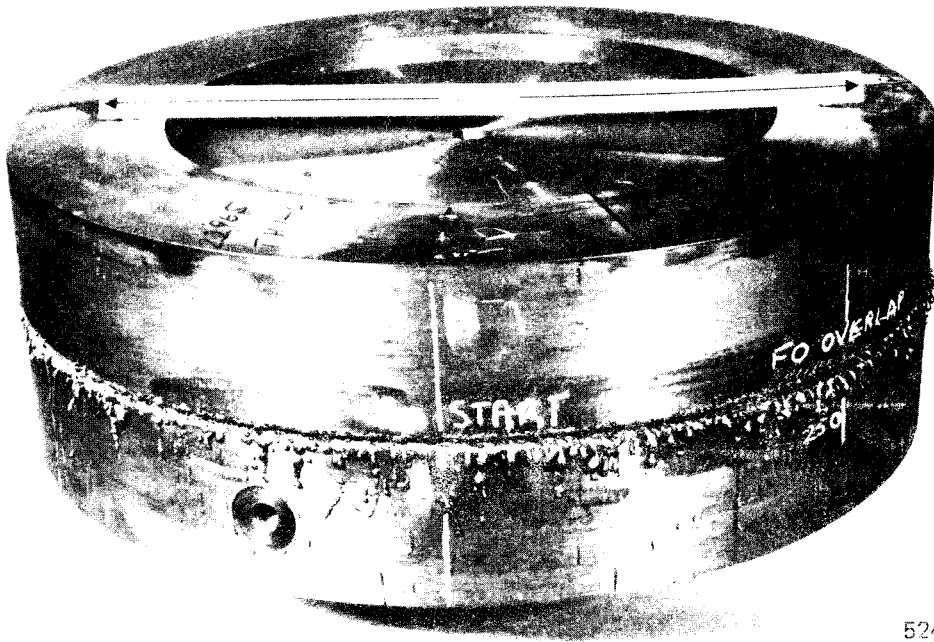
Fig. 18. General view of simulated lid assembly as-welded.
