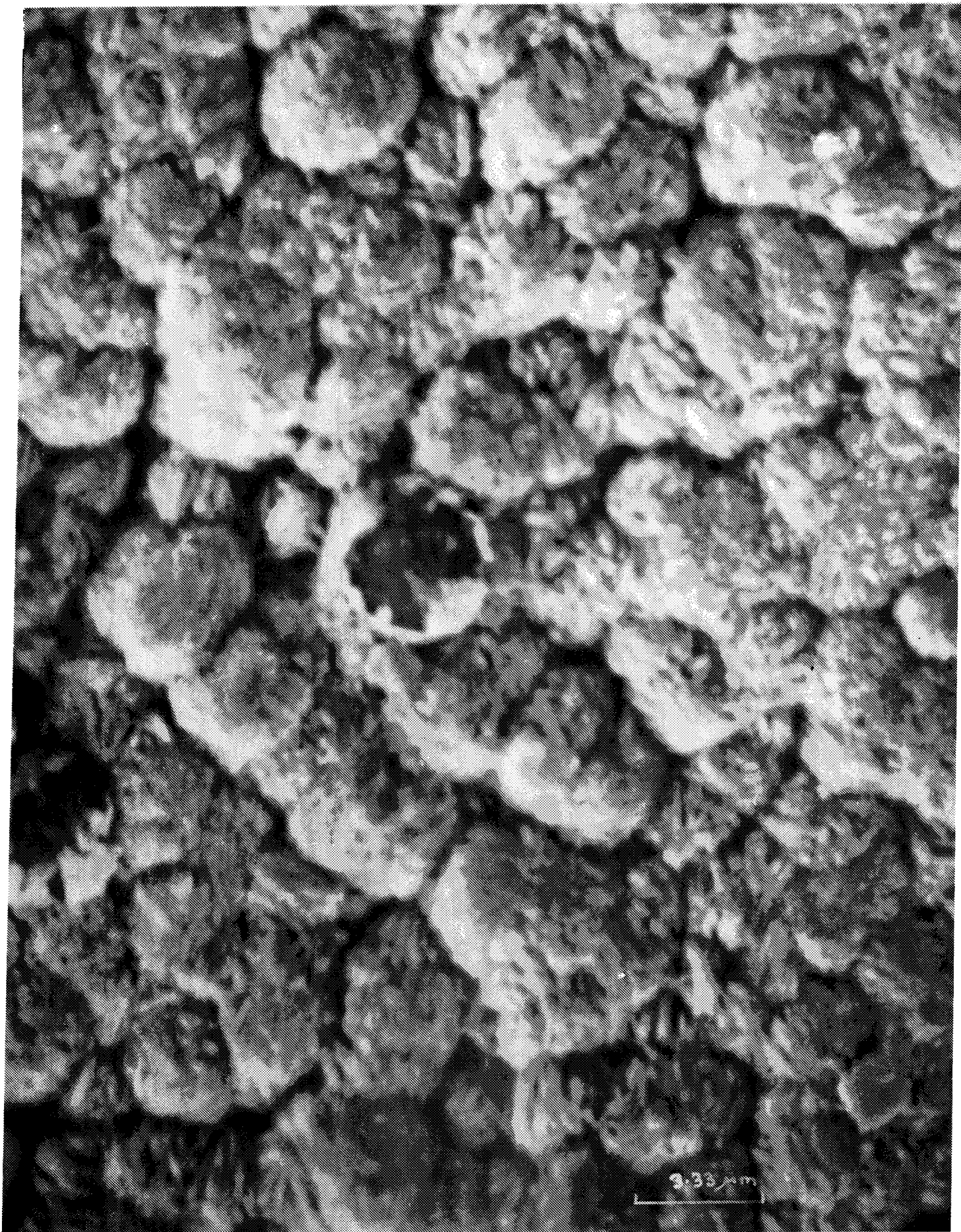
Fig. 2b SEM-photo of Al 2 O 3 autoclaved in water at 310°C for 24 h. Surface treated by 5M HCl before autoclaving.
