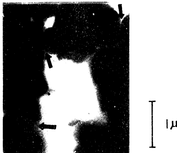
Fig. 2. Clay-sized particles in Cerithium limestone connected and covered by calcium carbonate cement.
