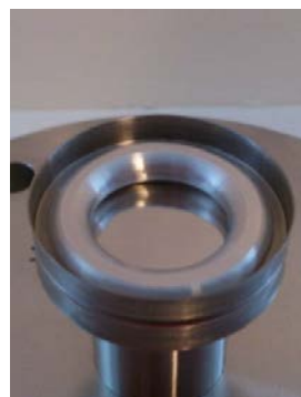
Figure 3-5. Sketch of sealing ring of the palladium membrane (left) and photographs of the installation (right).
