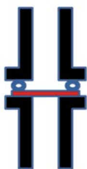
Figure 3-5. Sketch of sealing ring of the palladium membrane (left) and photographs of the installation (right).
