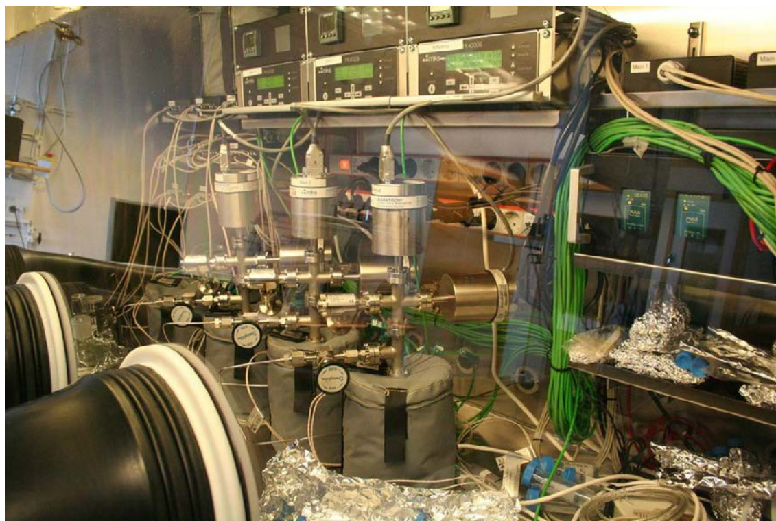
Figure 3-3. Interior of the glove box with three connected containers (Main 1, Reference 1, Reference 2).
