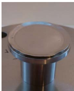
Figure 3-5. Sketch of sealing ring of the palladium membrane (left) and photographs of the installation (right).
