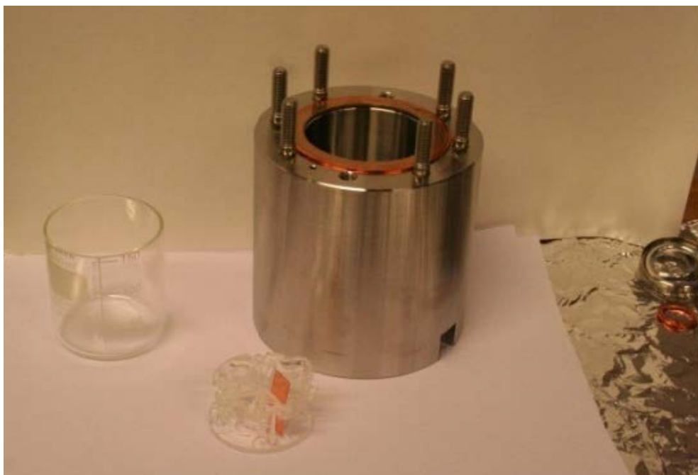
Figure 2-5. The reaction chamber with beaker and insert holder with an inserted copper plate.
