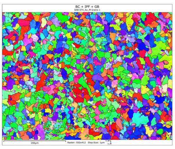
*Figure A-29.* Specimen ST4 in axial direction. Mid position. Lower magnification EBSD analysis showing the grain structure.
