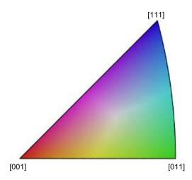
Figure 3-4. Inverse pole figure (IPF) colour key.
