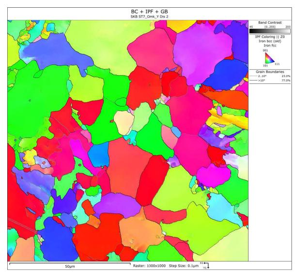
*Figure A-23.* Specimen ST7 in circumferential direction. Close to outer surface. Higher magnification EBSD analysis for dislocation analysis.
