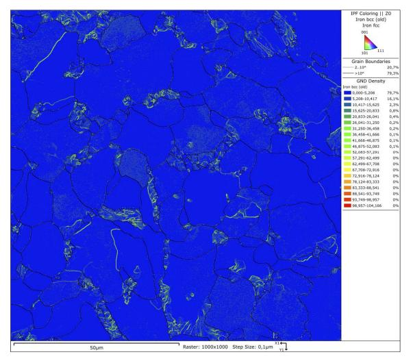
*Figure 3-7.* EBSD map at high magnification for dislocation density (GND) analysis. The areas with high GND corresponds to the perlitic areas in the material. GND analysis with Kernell size  $3 \times 3$  and  $5^{\circ}$  threshold for sub-grains.
