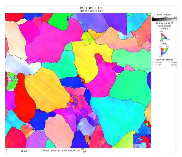
Figure A-47. ST4 circumferential direction, outer surface.
