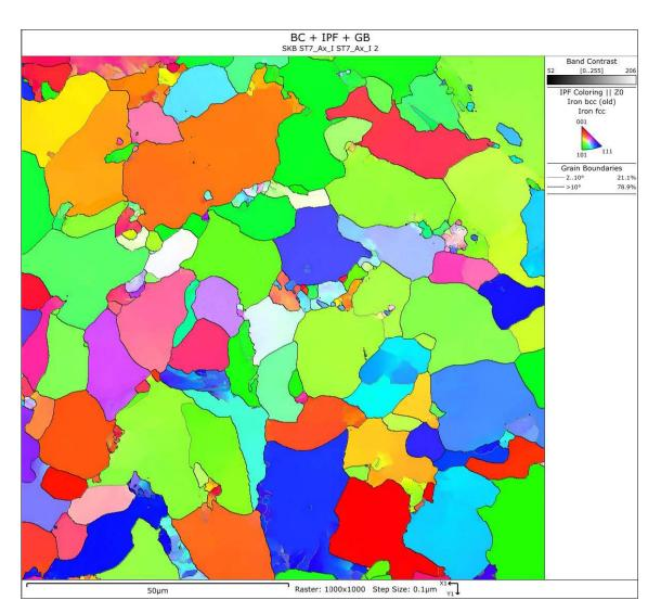
*Figure A-3.* Specimen ST7 in axial direction. Close to inner surface. Higher magnification EBSD analysis for dislocation analysis.
