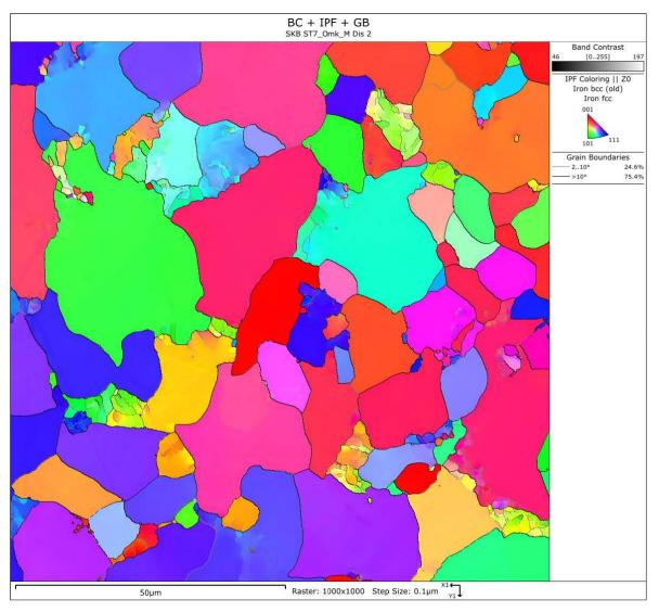
*Figure A-19.* Specimen ST7 in circumferential direction. Mid position. Higher magnification EBSD analysis for dislocation analysis.
