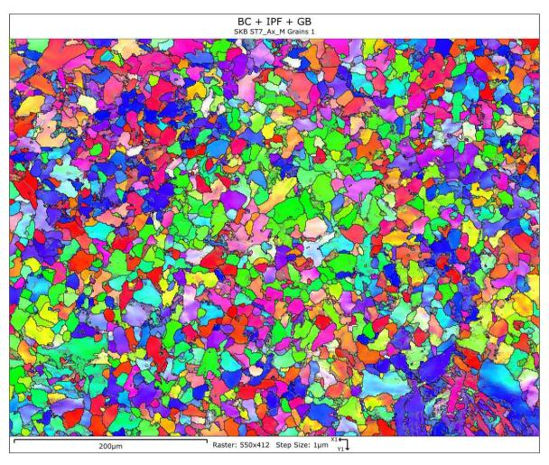
*Figure A-5.* Specimen ST7 in axial direction. Mid position. Lower magnification EBSD analysis showing the grain structure.
