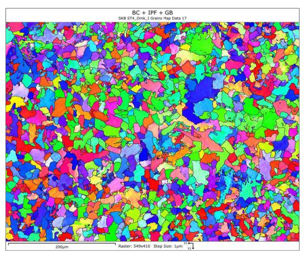
*Figure A-37.* Specimen ST4 in circumferential direction. Close to inner surface. Lower magnification EBSD analysis showing the grain structure.
