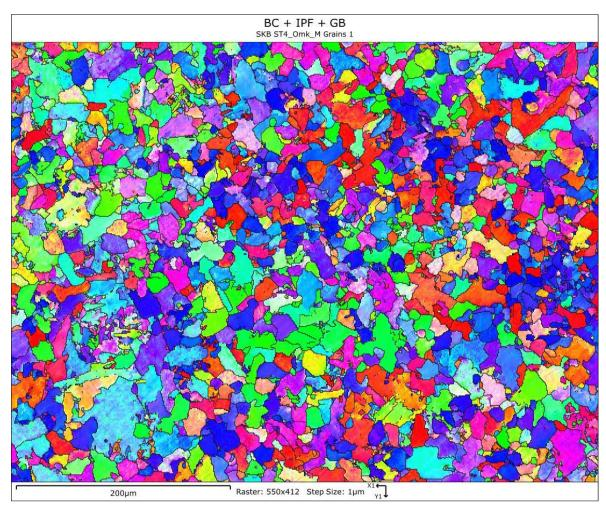
*Figure A-41.* Specimen ST4 in circumferential direction. Mid position. Lower magnification EBSD analysis showing the grain structure.
