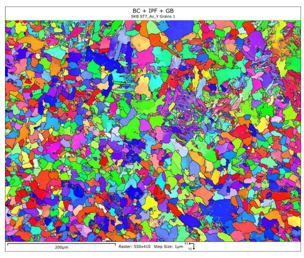
*Figure A-9.* Specimen ST7 in axial direction. Close to outer surface. Lower magnification EBSD analysis showing the grain structure.
