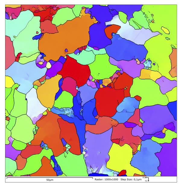
**Figure 3-6.** EBSD map at high magnification for dislocation density (GND) analysis. Colours according to crystal orientations by IPF colour key. Grain boundaries  $\geq 2^{\circ}$  thin black lines and grain boundaries  $\geq 10^{\circ}$  thick black lines.
