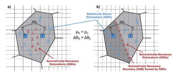
Figure 1-1. Geometrically necessary dislocations (GND) vs statistically stored dislocations (SSD).
