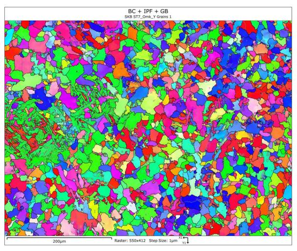
*Figure A-21.* Specimen ST7 in circumferential direction. Close to outer surface. Lower magnification EBSD analysis showing the grain structure.
