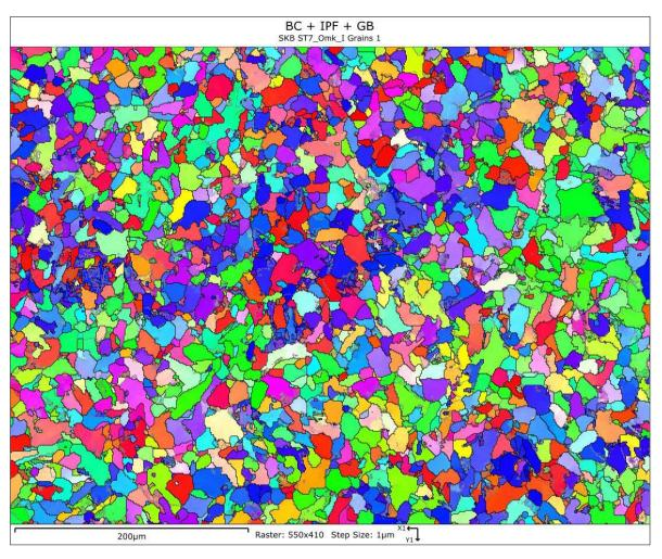
*Figure A-13.* Specimen ST7 in circumferential direction. Close to inner surface. Lower magnification EBSD analysis showing the grain structure.
