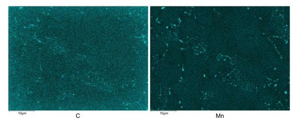
*Figure 3-2. EDS mapping analysis showing carbon and manganese distribution of the same area as in Figure 3-1. Cementite contains more carbon and manganese compared to the matrix. Bright areas contains more C or Mn compared to dark areas.*
