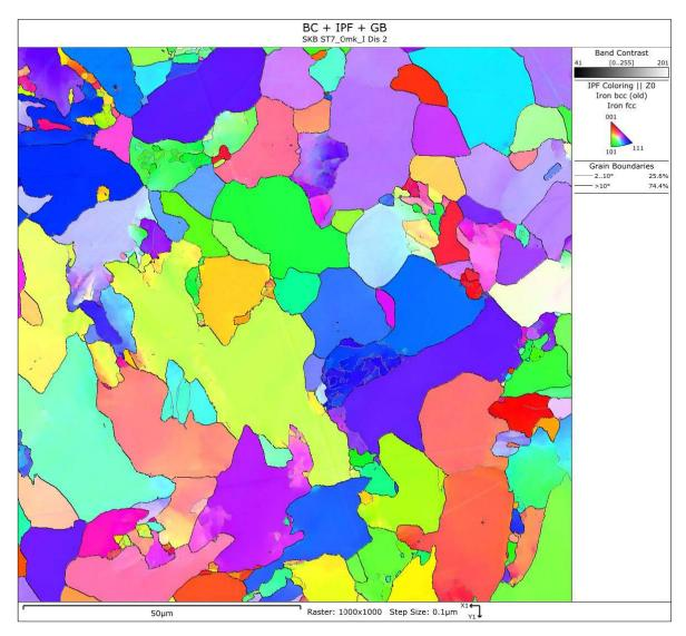
*Figure A-15.* Specimen ST7 in circumferential direction. Close to inner surface. Higher magnification EBSD analysis for dislocation analysis.
