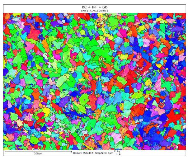
*Figure A-25.* Specimen ST4 in axial direction. Close to inner surface. Lower magnification EBSD analysis showing the grain structure.
