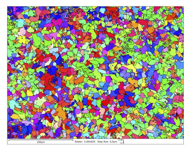
*Figure 3-3. EBSD* map at low magnification for grain size analysis. Colours according to crystal orientations by IPF colour key. Grain boundaries  $\geq 2^{\circ}$  present as black lines.
