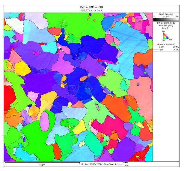
*Figure A-11.* Specimen ST7 in axial direction. Close to outer surface. Higher magnification EBSD analysis for dislocation analysis.
