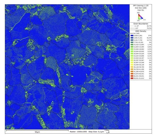
Figure 3-8. Same plot as in Figure 3-7, but the GND analysis was performed with 2° threshold for sub-grains.
