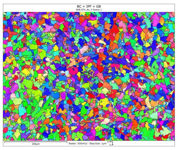
*Figure A-33.* Specimen ST4 in axial direction. Close to outer surface. Lower magnification EBSD analysis showing the grain structure.
