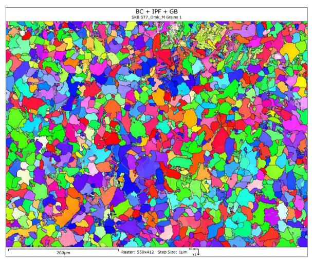
*Figure A-17.* Specimen ST7 in circumferential direction. Mid position. Lower magnification EBSD analysis showing the grain structure.
