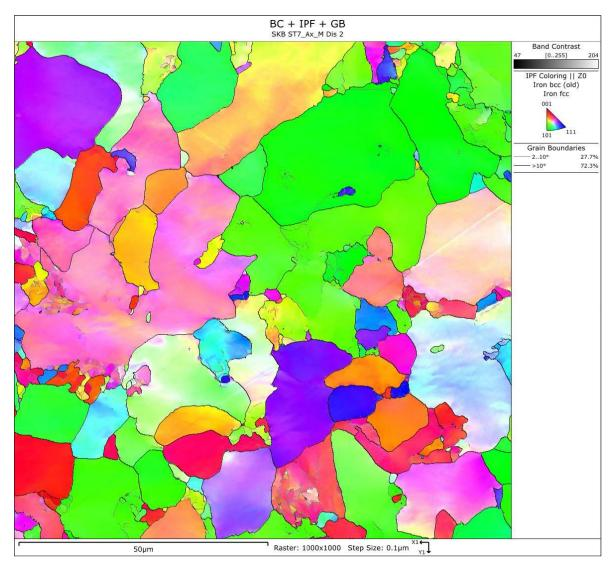
*Figure A-7.* Specimen ST7 in axial direction. Mid position. Higher magnification EBSD analysis for dislocation analysis.
