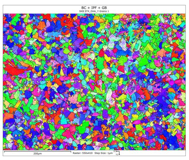
*Figure A-45.* Specimen ST4 in circumferential direction. Close to outer surface. Lower magnification EBSD analysis showing the grain structure.
