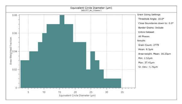
Figure 3-5. Grain size distribution for material ST7 in axial direction close to the inner surface.
