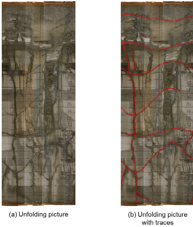
Figure 5-4. Unfolding picture of bentonite surface of dismantled bentonite column from KO0018G bore.
