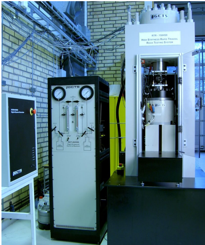
Figure 3-2. Rock testing system. From left: Digital controller unit, pressure cabinet (used for triaxial tests) and load frame. The PC with the test software (not shown in the picture) is placed on the left hand side of the controller unit.
