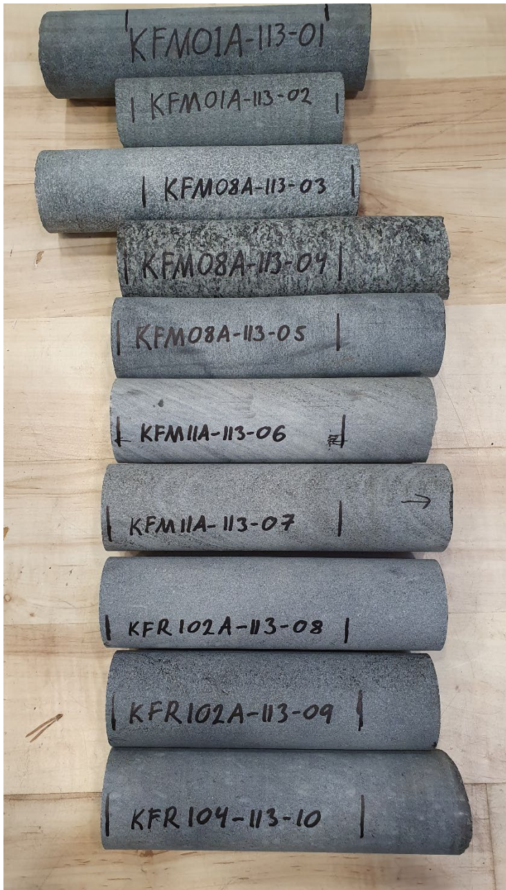
Figure 2-1. Layout for cutting the uniaxial compression test specimens. The order of the specimens in the image follows, from top to bottom, Table 2-3.
