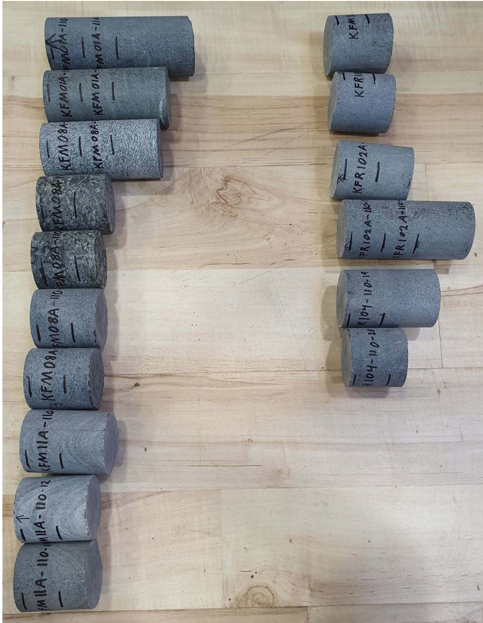
Figure 2-2. Layout for cutting the indirect tensile test specimens. The order of the specimens in the image follows, from top to bottom, Table 2-2.
