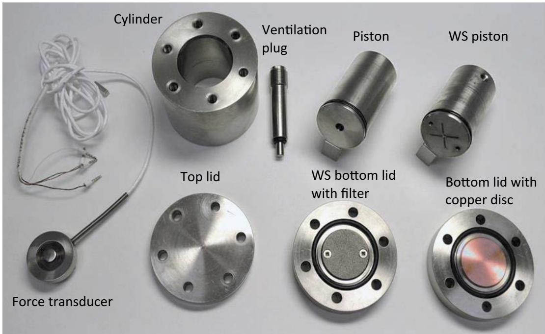
Figure 3-7. All the parts included in a test cell. The parts in contact with the bentonites were made of titanium. See text for details. WS = water saturation (Bengtsson et al. 2017a).
