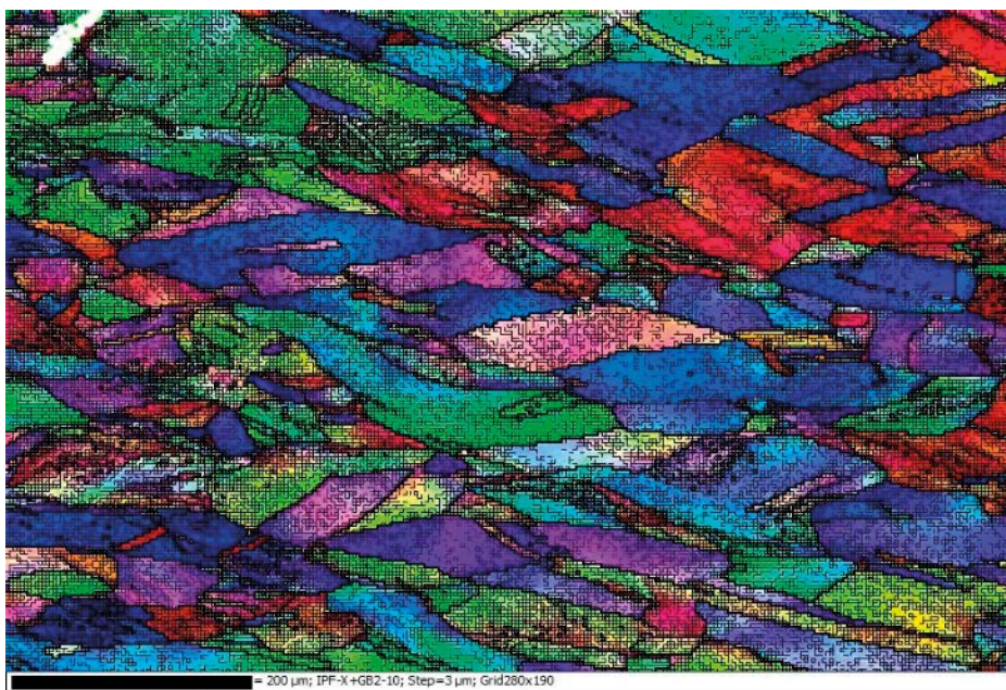
Figure 3-12. 175 °C, 6 months, 3 \mu\text{m} step length. The deformed substructure is very clearly still present, despite the long ageing duration at 175 °C. 200 \mu\text{m} scale bar.
