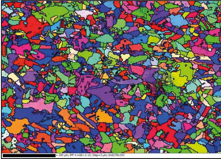
Figure 3-21. 250 °C, 6 months. The microstructure is completely recrystallized. Some deformation remained from specimen preparation. 200 \mu\text{m} scale bar.
