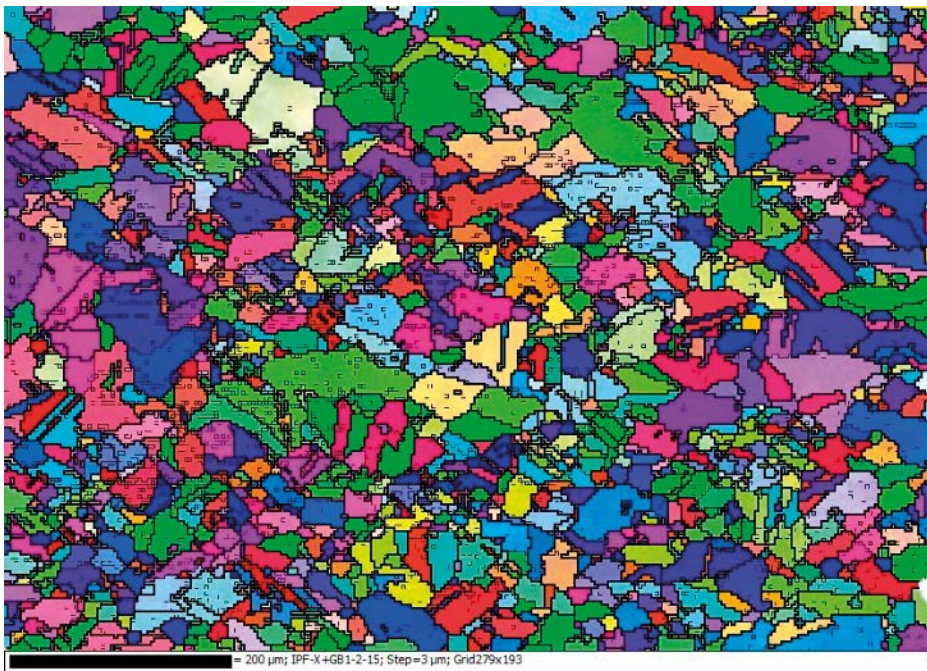
Figure 3-22. 250 °C, 12 months. Some deformation remained from specimen preparation. However, the specimen is completely recrystallized. 200 \mu\text{m} scale bar.
