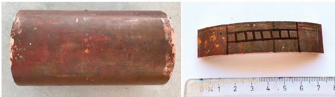
Figure A-16. Left: Condition of the reference pipe sample as received. Right: Positions of reference pipe samples that were extracted for H and O analysis.
