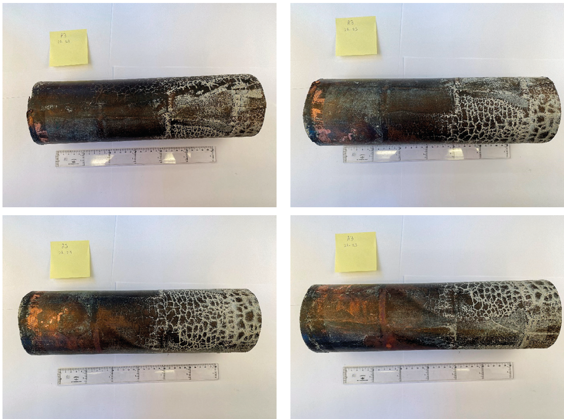
Figure A-12. Pipe sample A3 as-received, photographed at 0°, 90°, 180°, 270° rotation.
