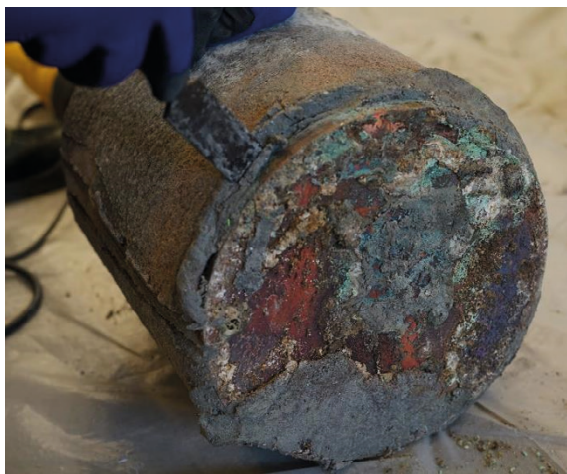
Figure 3-1. Appearance of the bottom plates immediately after retrieval. Note the blue-green deposits. Upper left: Bottom plate of A3 when it was still surrounded by rock. Lower left: Bottom plate of A3 when the pipe was still embedded in the bentonite. Right: Bottom plate of S2.
