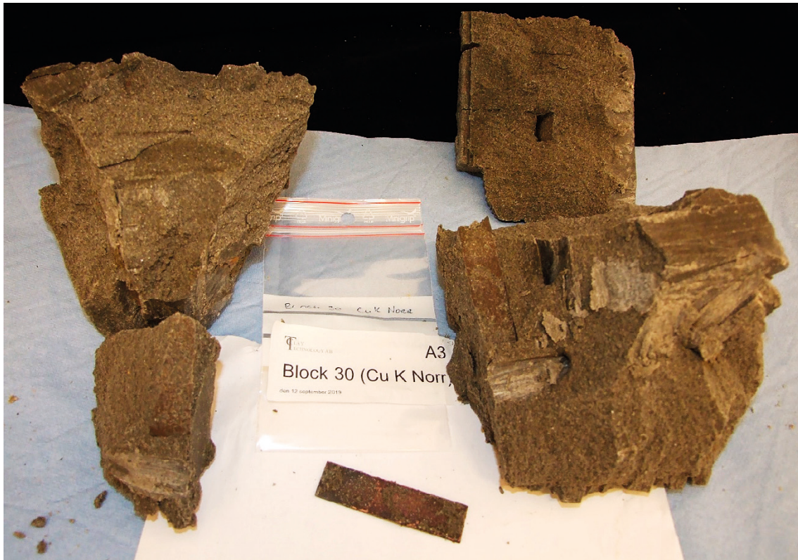
Figure A-4. Corrosion coupon A3/K with surrounding bentonite clay.
