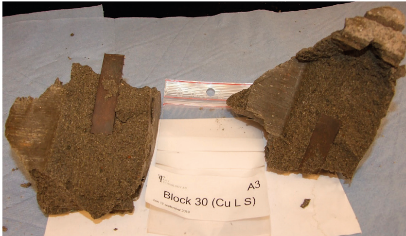
Figure 3-5. Corrosion coupon A3/L with surrounding bentonite clay.
