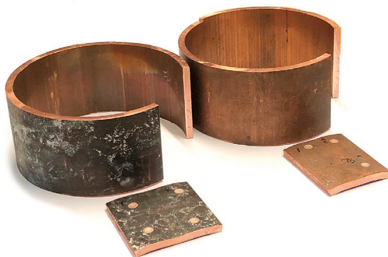
Figure H-2. The pipe sections (left: A3, right: S2) and corresponding samples for GDOES analysis.
