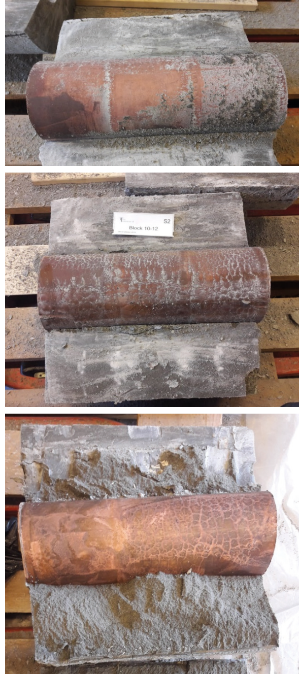
Figure 3-3. Appearance of the copper pipes in LOT A3 and S2 immediately after uncovering the pipes.
