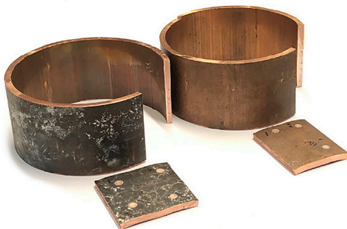
Figure 2-1. Sections of pipe A3 (left) and S2 (right) for GDOES analysis. The small circles visible on the surfaces are the spots of analysis.
