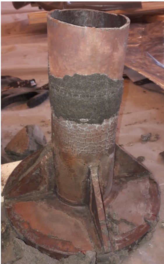
Figure 3-2. Appearance of the lower part of the copper pipes immediately after retrieval.
