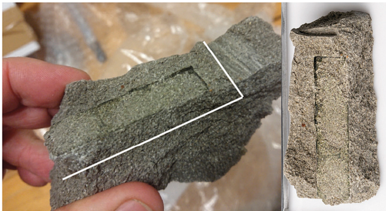
Figure 3-25. Sample “30 Cu K N” from block 30 of LOT A3, before and after trimming. All bentonite at 10 mm distance from the copper coupon was included in the final sample.
