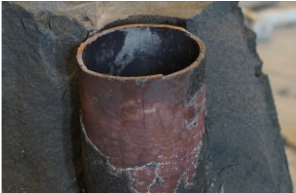
Figure 3-4. Appearance of the interior of the copper pipes in LOT A3 and S2 immediately after retrieval.
