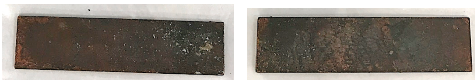
Figure A-9. Corrosion coupon S2/O, left: milled side; right: polished side.
