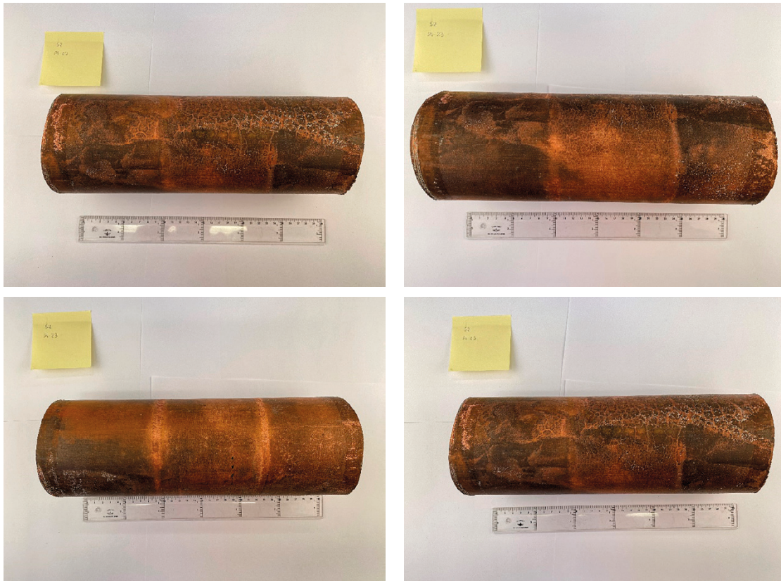
Figure A-14. Pipe sample S2 as-received, photographed at 0°, 90°, 180°, 270° rotation.
