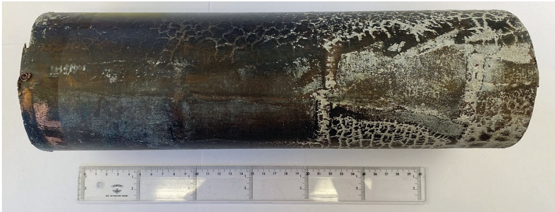
Figure 3-7. Pipe sample A3 in as-received condition.
