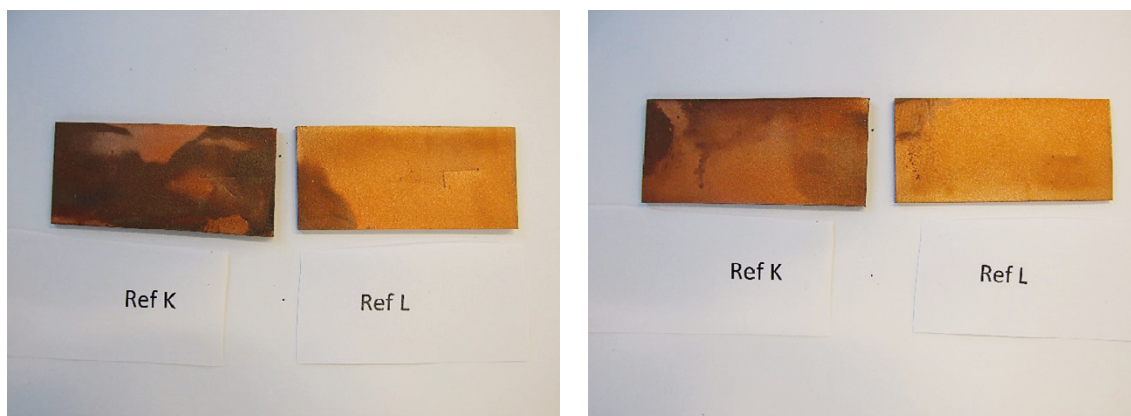
Figure A-11. Reference coupons K and L as-received, left: milled side, right: polished side.
