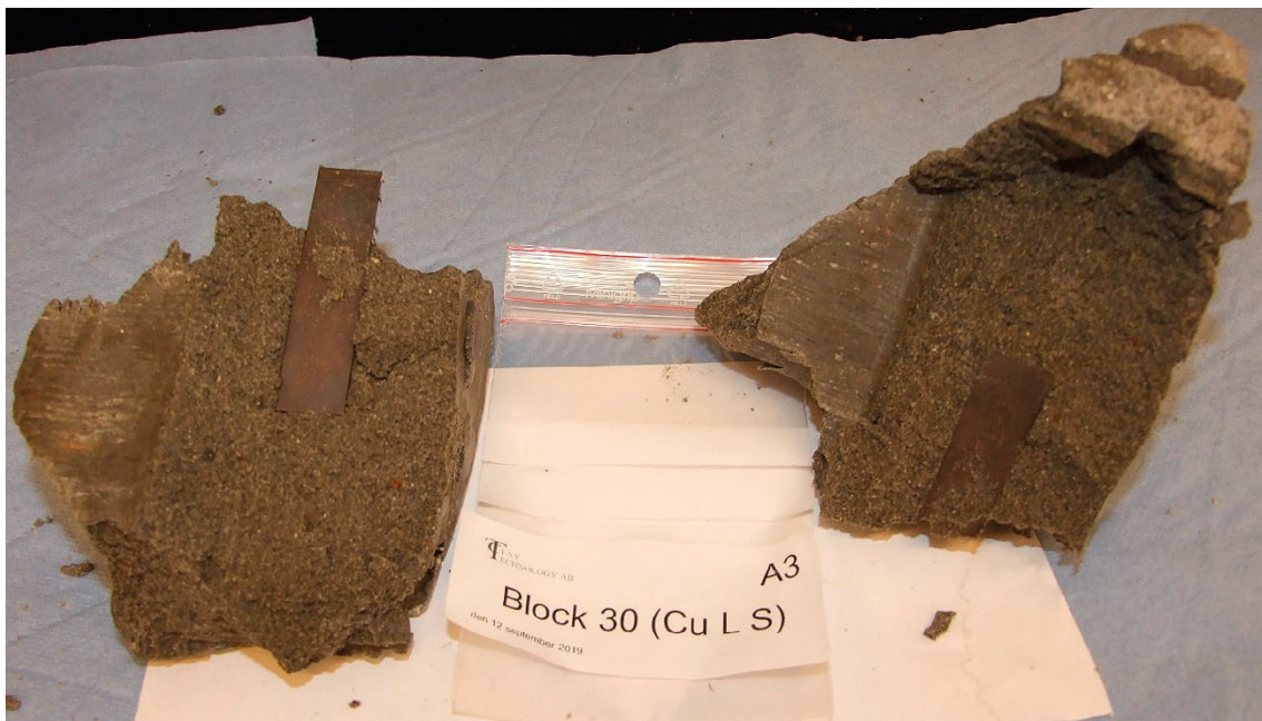
Figure A-5. Corrosion coupon A3/L with surrounding bentonite clay.
