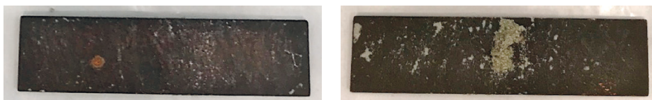
Figure A-10. Corrosion coupon S2/P, left: milled side; right: polished side.
