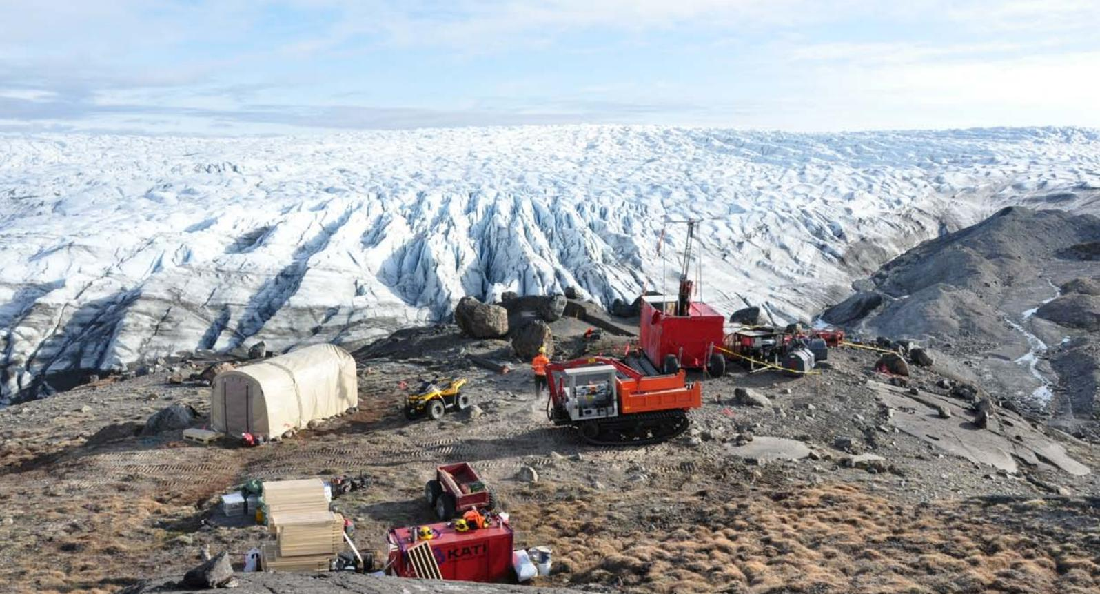
*Borehole drilling to repository depth to study the water chemistry and pressure gradient.*
