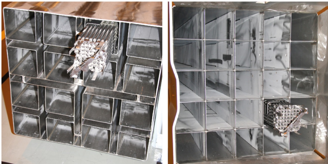
Figure 4-1. To the left is a normal storage canister that holds 16 assemblies of BWR type and to the right a compact storage canister that holds 25 assemblies of BWR type.
