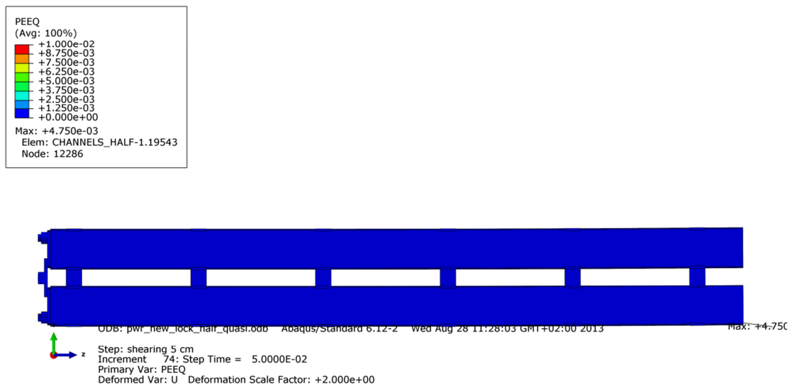
Figure A6-10. Plot shows equivalent plastic strain (PEEQ) for the steel channel tubes after 5 cm shearing.
