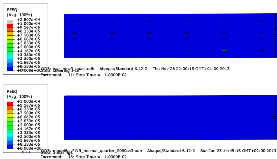
Figure A8-9. Plot shows plastic equivalent strain (PEEQ) for the insert after 5 cm shearing for detailed PWR model (upper) and the reference PWR model (lower).
