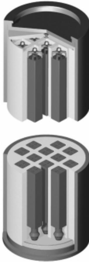
**Figure 1.** Exploded view of SKB canister for spent nuclear fuel.
