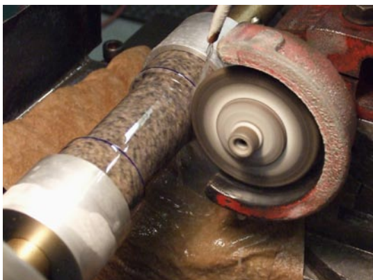
Figure 1. Grinding Specimen with Lathe Tool-Post Grinder.
