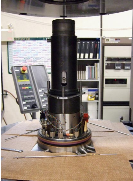
Figure 4-3. Split-Grip Direct Tensile Strength Test Assembly set up in MTS Test System.
