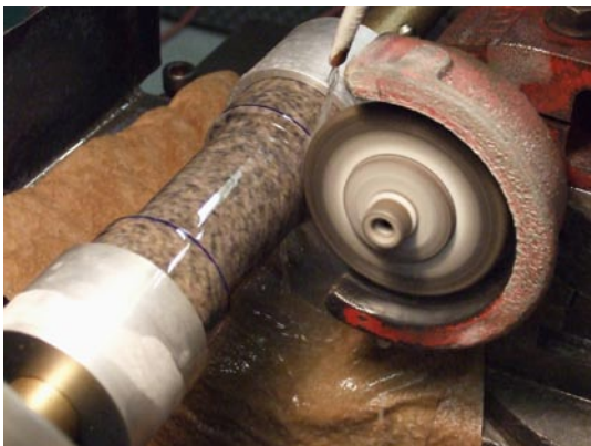
Figure 4-1. Grinding Specimen with Lathe Tool-Post Grinder.
