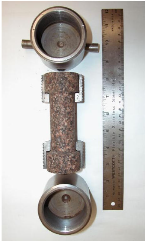
Figure 2. Split-Grip Direct Tensile Strength Test Assembly (typical).
