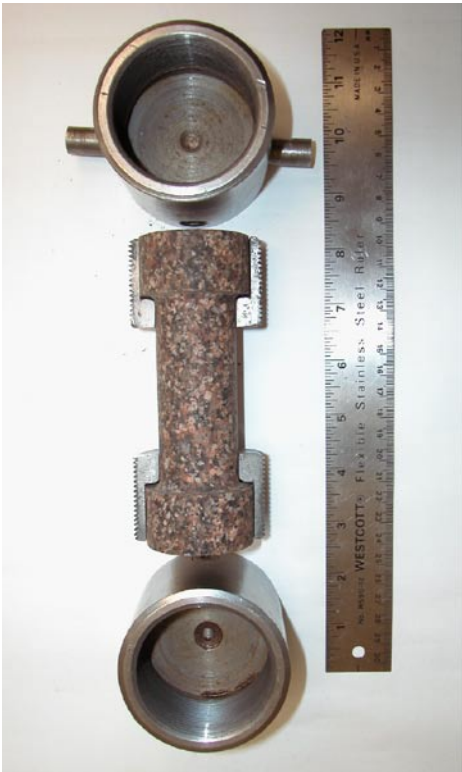
Figure 4-2. Split-Grip Direct Tensile Strength Test Assembly (typical).
