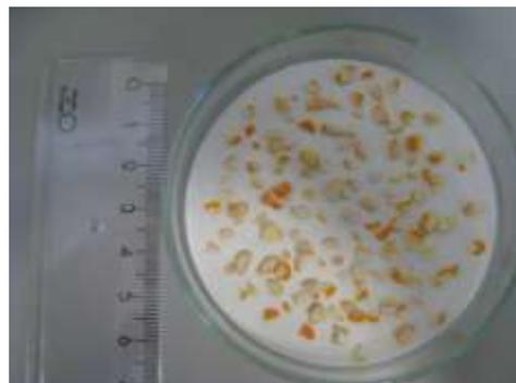
Figure 1. Fragments of the  $\text{ThO}_2$  pellet made in Sheffield. Note the bright orange colour.
