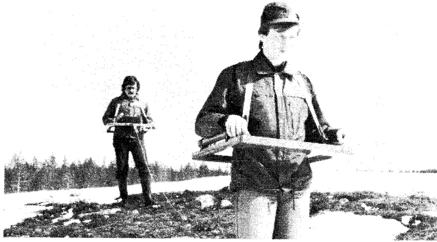
Figure 2-5. Slingram (Horizontal Loop EM), frequency 18 kHz, coil separation 60 m
