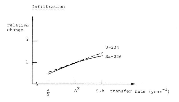
The relative changes of the doses from uranium-234 and its daughter product radium-226 when the rate of the infiltration in the soil reservoir is varied. The reference values (A) are  $1 \cdot 10^{-3}$  year and  $4.5 \cdot 10^{-3}$  year for uranium and radium respectively.
