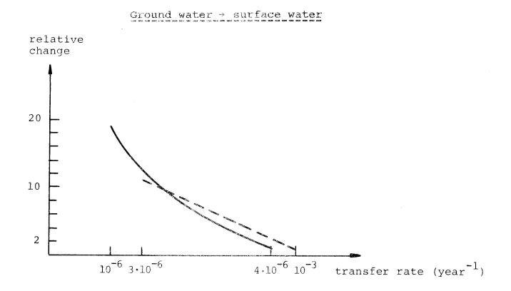
The relative changes of the doses for uranium-234 and radium-226 when the transfer rate from the groundwater to the surface water is changed. The reference values are  $10^{-9}$  year and  $4 \cdot 10^{-4}$  year for uranium-234 and radium-226 respect-ively.
