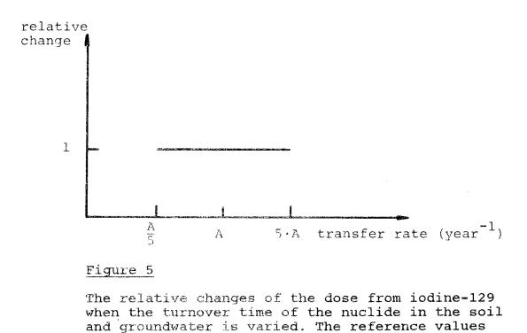
A are groundwater  $\rightarrow$  surface water 0.2 year<sup>-1</sup> groundwater  $\rightarrow$  soil 0.1 year<sup>-1</sup> As for the case of varying transfer based upon irrigation, the influence of the resulting dose is totally negligible
