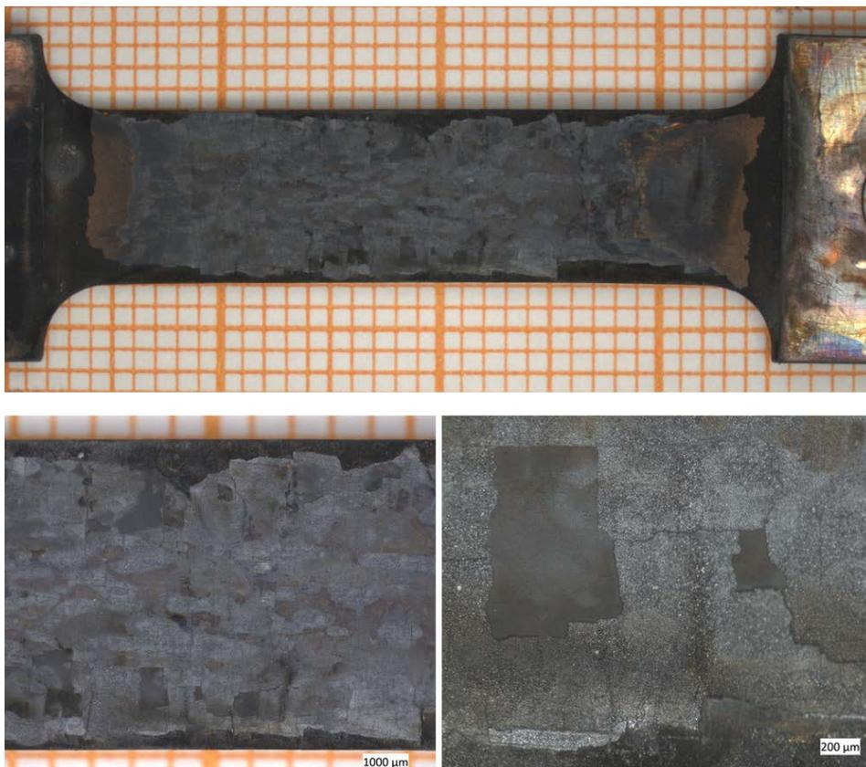
**Figure 5-9.** The surface appearance of the creep sample after sulphide test 1.
