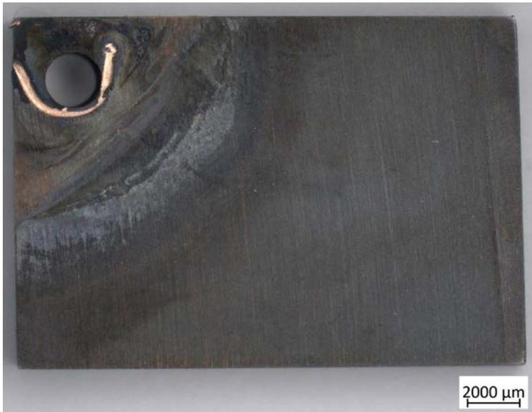
*Figure 5-15. The surface appearance of the coupon sample after sulphide test 2.*
