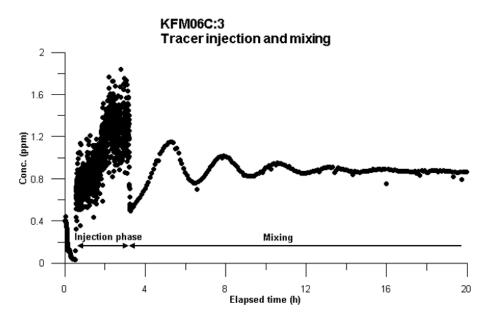
Figure 4-1. Injection phase and mixing in KFM06C:3.
