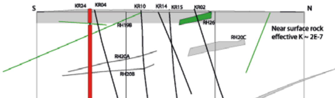
Figure A4-5. Options for representation of near surface rock in KR24 pump test simulation models.
