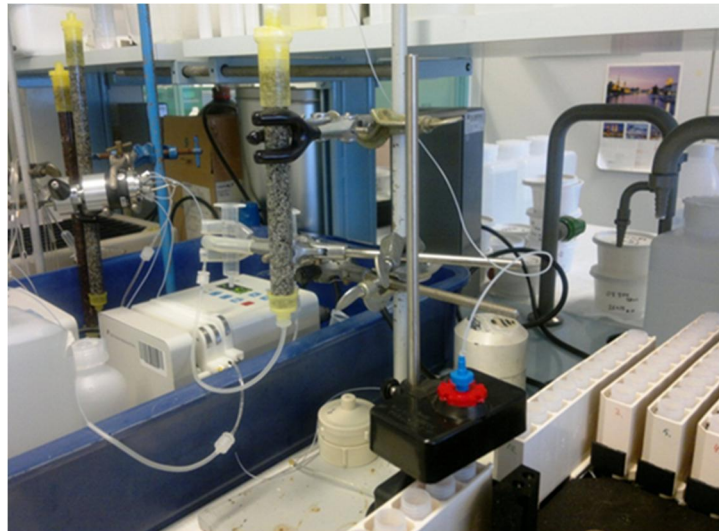
Figure 2. The experimental set-up for the crushed rock and drill core column experiments.
