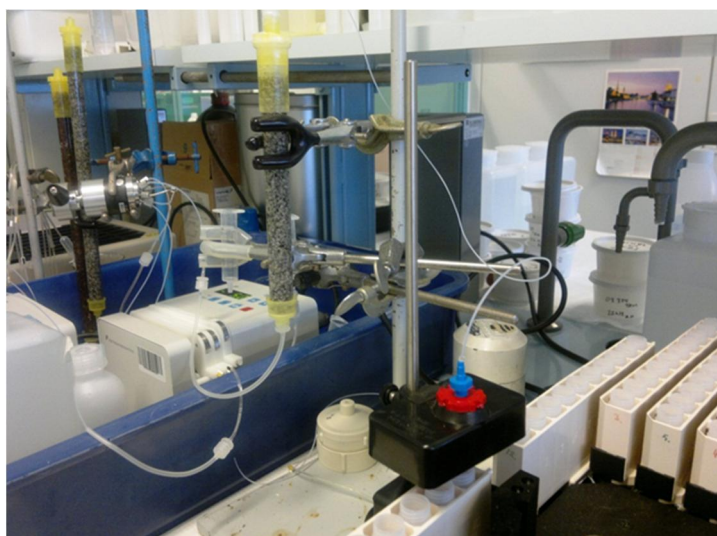
Fig. 2. The experimental set-up for the fracture and crushed rock column experiments.
